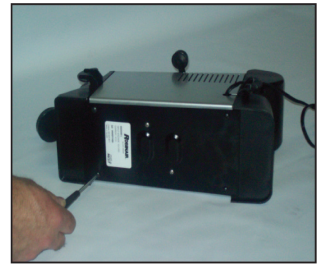
Illustration 5.3 - Remove the Four Pan Philips Screws
