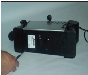
Illustration 3.2 - Remove Six Screws at the Base Plate
