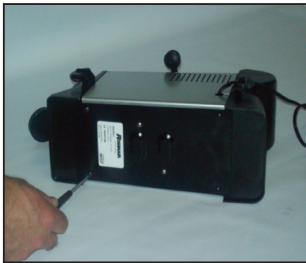
Illustration 4.17 - Install Four Pan Phillips Screws
