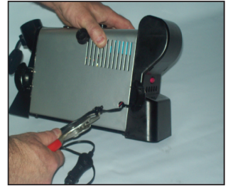
Illustration 5.2 - Remove Strain Relief
