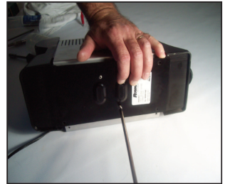
Illustration 3.11- Tighten Two Center Screws
