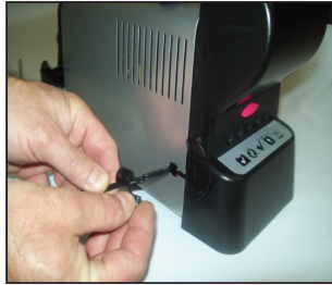
Illustration 4.18 - Strain Relief on Power Cord
