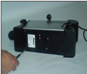
Illustration 4.3 - Remove Four pan Phillips Screws
