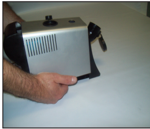
Illustration 4.4 - Remove Main Metal Body Housing
