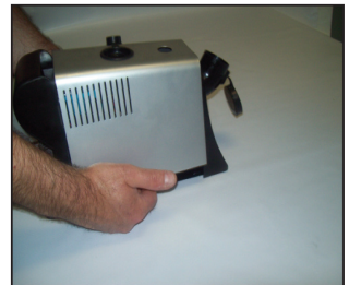
Illustration 5.4 - Remove Main Metal Body Housing
