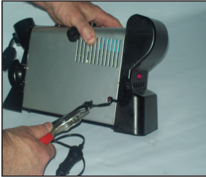
Illustration 4.2 - Remove Strain Relief
